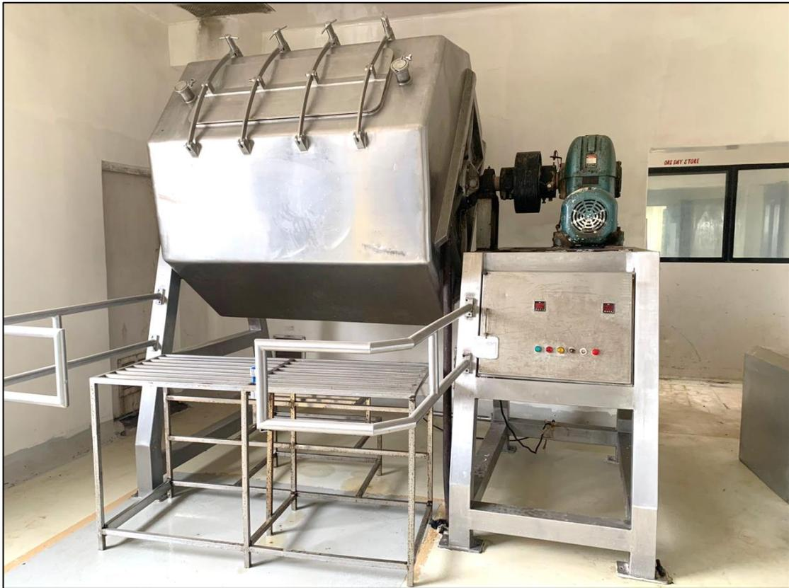
*Blender Machine for Dry Granules Mixer*
