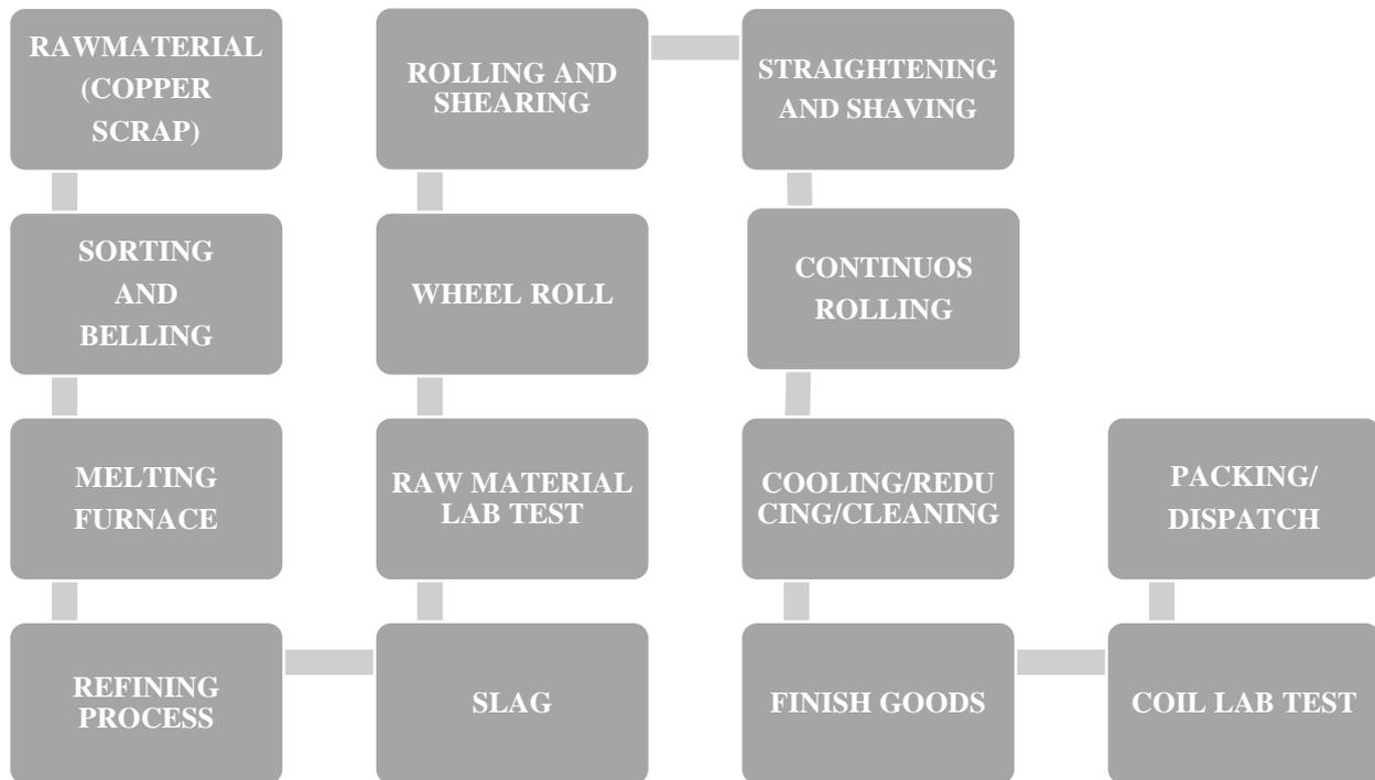
1. **RAW MATERIAL (COPPER SCRAP):** The production process begins with the procurement of copper scrap as the raw material for wire rod manufacturing.
