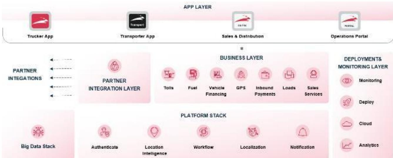
**Application layer:** This layer interfaces with truck operators, and other business stakeholders including shippers, channel partners and internal teams. These applications are built by in-house teams using a combination of multiple front-end technologies.
